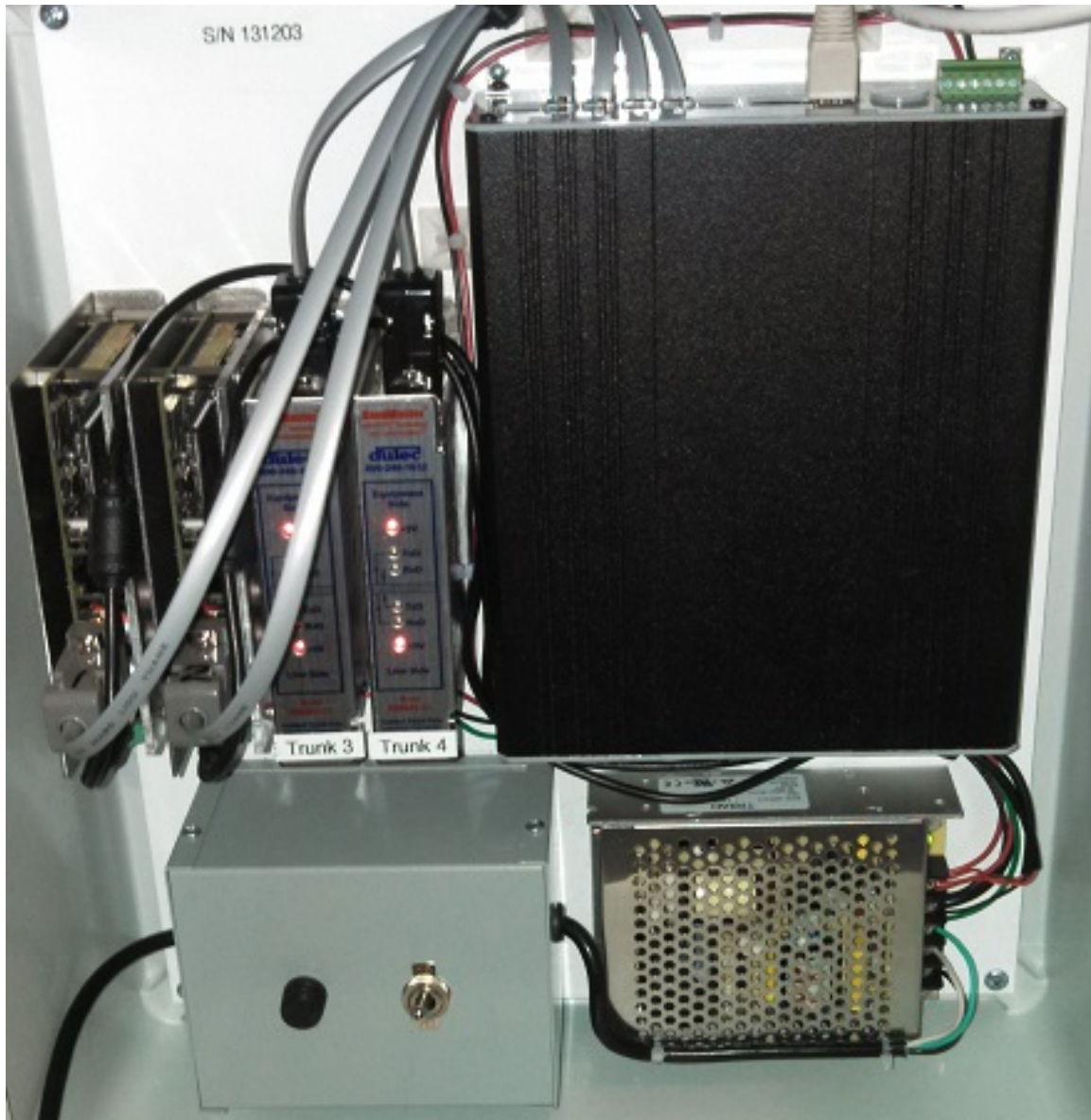
Picture 1.3C, Gateway Overview and Identification, with two Wireless Co-Processors
